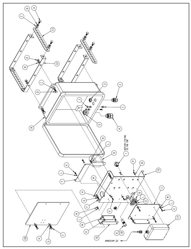
Figure 1. WLVEH Outdoor Enclosure Exploded Assembly Diagram
